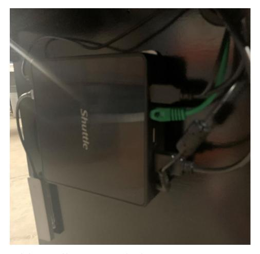
Pro tables will come with the computer mounted. WHC tables will need the computer attached to the mount. Both tables will require wires to be plugged in. Attach all wires coming out of the side of the cabinet to the computer. Unpack and attach the mouse and keyboard.
