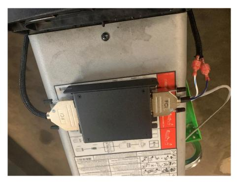
Plug on the Stingray module to the wire coming from the table. There are 2 wires that will plug in to the loom. Match the colors when connecting. The serial plug will plug into the module then the power unit.
