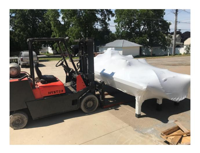
Care should be taken when unloading your table as not to damage it by collisions with the lift or objects in the area. Position your forks slightly left of center under the table on the side without the track. Fork extensions are highly recommended. Lift taking notice that the load is even, if the table is heavy to one side reposition the lift. Place the table in its area.
