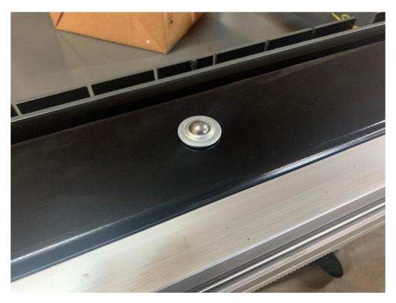
Insert supplied rollers into the holes along the rails.
