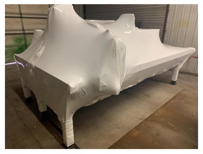
Your Boss Plasma table will come securely shrink wrapped and safe from the elements. Care should be taken when opening the wrap. Use short mindful cuts opening while checking for wires and avoiding scratching or marring. Special care needs to be taken on the track side of the table due to the presence of many wires.
