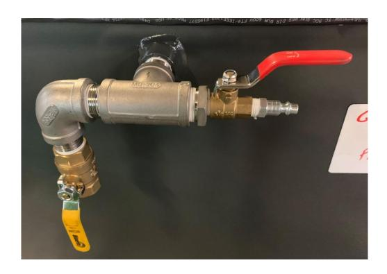
Make sure the valves on the end of the table are open to allow air to bleed out when filling. Under the table, check that the valve is in the horizontal (closed) position.
