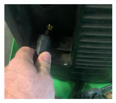
Plug the ground into the twist lock port on the power unit.
