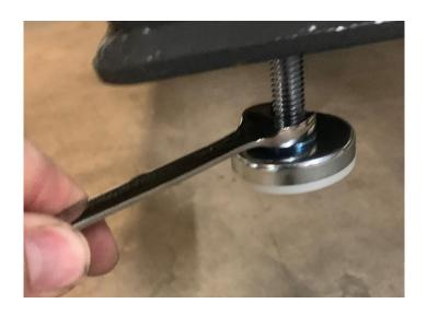
Using a level, check all sides. Make necessary adjustments to the feet with a 9/16" wrench to make the table level.
