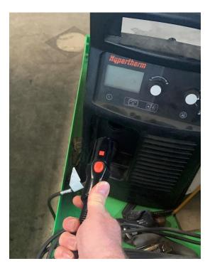
Plug the torch lead from the table into the power unit.
