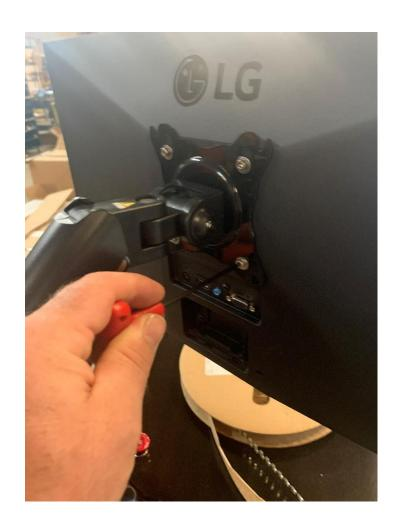
Your monitor will come prewired. Mounting screws will be in the back of the monitor. Simply attach to the mount.
